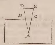
Each fide A D, and A E, being one, the points B C, being in stead of severall props or fulciments; the weight to be moved at A, and the power that should move it, being applyed to the top D E, by the force of some stroake or blow: as Aristotle hath explained the severall parts of this faculty. But now, because this instrument may be so used that the E 3 point
